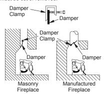
Figure 3 - Attaching Damper Clamp
